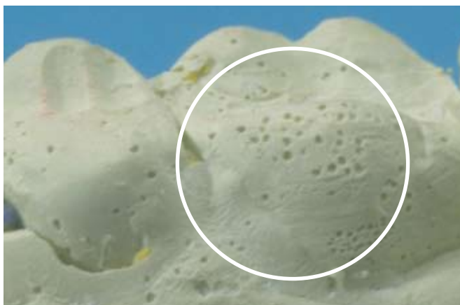
Stone Model with Hydrogen Evolution Voids
