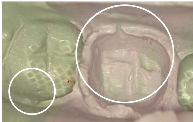
Void Caused by Syringe Technique
